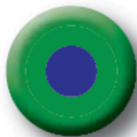
Drinking Water Cold
