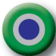
Demineralised Water Cold
